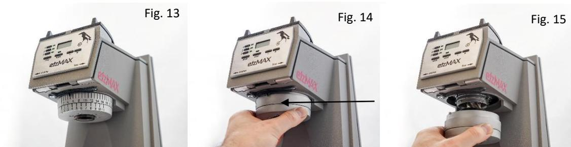
Remove adjustment by turning the macro-ring counterclockwise (Fig. 14) until you feel no more resistance. Slowly pull it downwards and out (Fig. 15).
