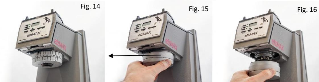
Remove adjustment (11) by turning the macro-ring counterclockwise (Fig. 15) until you feel no more resistance. Slowly pull it downwards and out (Fig. 16).
